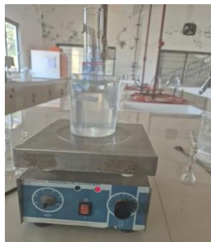
FIGURE 2: INVITRO DRUG RELEASE SETUP
