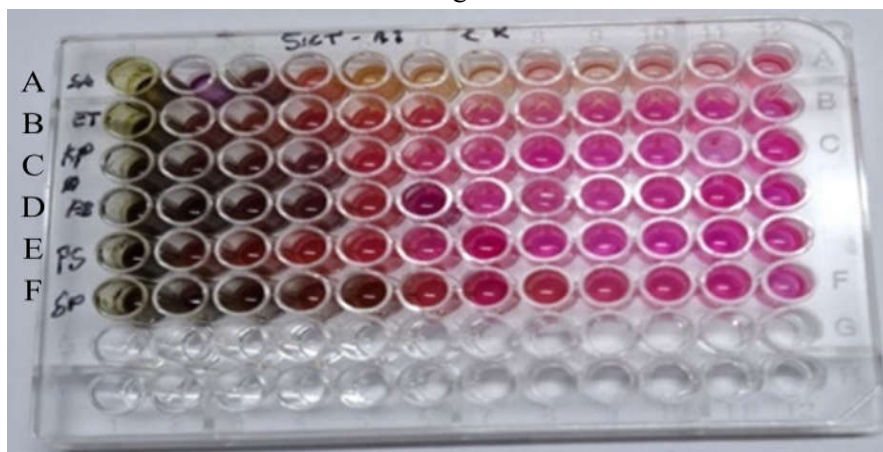
Figure 5: Determination of minimum inhibitory concentration (MIC) of Cocculus hirsutus extract using microdilution assay, showing visible color change indicative of microbial growth across tested concentrations.
